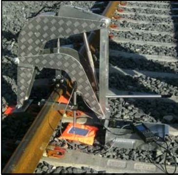
Output from the transducers are sent to the FW900
